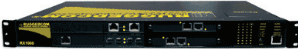
Figure 14. RuggedCom Ethernet Router
